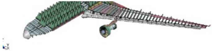
Figure 6-13. Finite element model of the Boeing 767-200ER.
